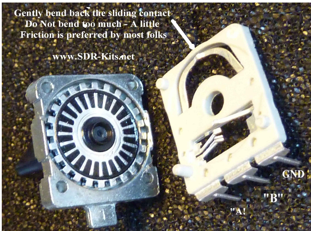
Appendix 1 - Fig 2 - Adjusting Click Stop Spring
