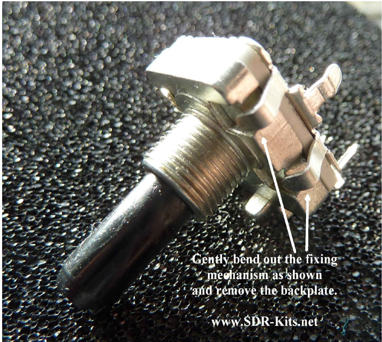
Appendix 1 - Fig 1 - Adjusting Click Stop Spring
