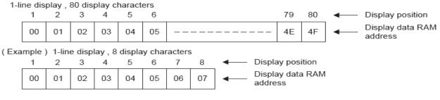
When the display shift operation is performed , the display data RAM's address moves as :
