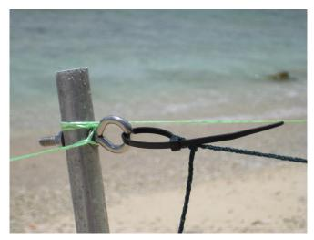
I was not prepared for an elevated radial system either (instead of insulators I was carrying a heavy bag of wire spikes for nailing ground radials to the ground). Plastic cable ties have been used as insulators. There was no sparking or burning when operating with 100w. I reckon as per Ohm law, for higher voltage insulation, two ties could be 'connected in serial'...
