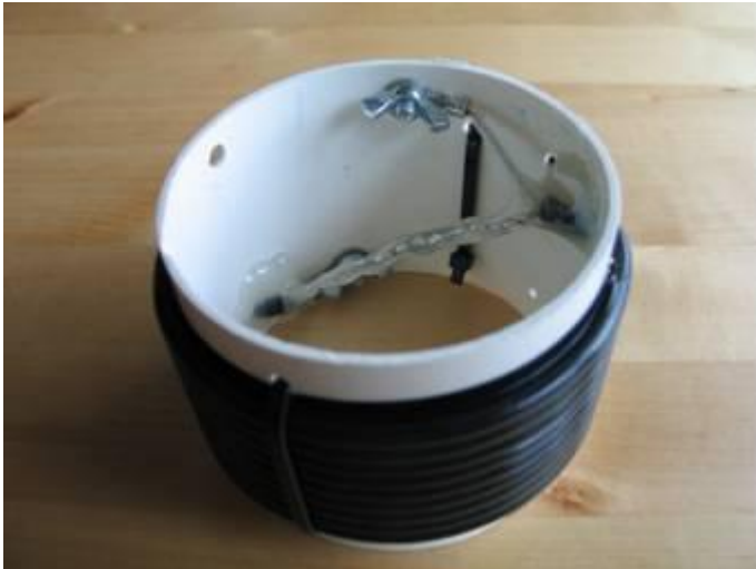
Fig.7. 80m band trap - 8.7w RG58 cable on 90mm diameter plumbing tube
