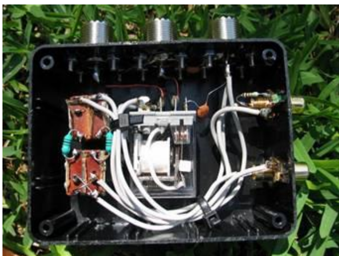
Fig. 13. The inside of the shack-end Beverage control box. Includes TX/RX antenna switching relay
