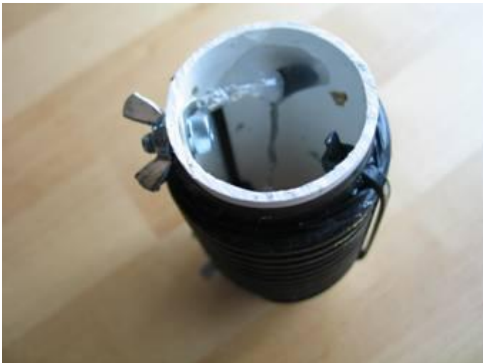
Fig.8. 40m band trap – 10.3w of RG58 cable on 43mm plumbing tube
